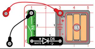
Build the circuit as shown, with the red & black jumper wires initially hanging loose. Turn on the switch (S1); the white LED (D6) will be off, because the air separating the ends of the jumper wires has very high resistance to electricity. Touch the loose ends of the jumper wires together and the LED will be very bright. Next, connect the loose ends of the jumper wires to the resistors (RV & R5) and the speaker (SP2), and see how bright the LED is.
