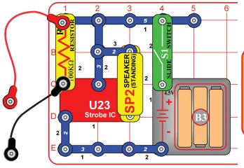
Long, narrow shapes have more resistance than short, wide ones, so different sounds are produced. The black core of pencils is graphite, the same material used in your resistors (R5 & RV).
