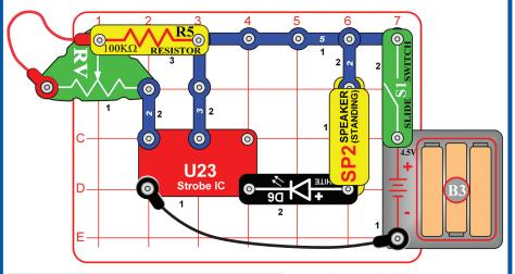
Turn on the slide switch (S1). The white LED should be flashing and you hear sound from the speaker (SP2). Move the lever on the adjustable resistor (RV) to adjust the flash rate and sound.
