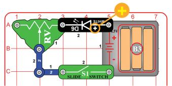
Turn on the switch (S1) and move the lever on the adjustable resistor (RV) to change the brightness of the white LED (D6).
