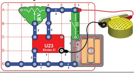
Build the circuit, connecting the speaker (SP2) with the red & black jumper wires as shown. Turn on the switch (S1) and adjust the tone of the sound using the adjustable resistor (RV). Most of RV's range will produce a buzzing sound, but part of it will produce an interesting tone. Try to make music with it.
