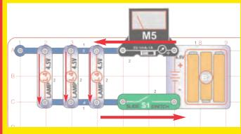
The three lamps are connected in parallel with one another. They are bright because each lamp gets the full battery voltage. The voltage pushes the current with equal force, because all are 4.5V, down each path.
