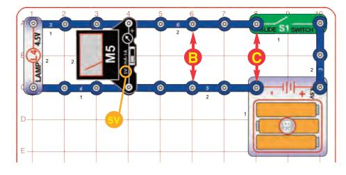
Build the main circuit and set the meter (M5) on the 5V setting. Turn on the slide switch (S1); the lamp (L4) lights and the meter (M5) measures the voltage from the batteries (B3).
