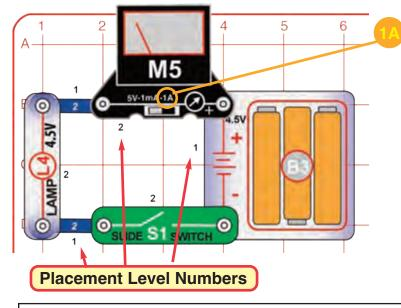
Build the circuit shown by placing all the parts with a black **1** next to them on the board first. Then, assemble parts marked with a **2**. Install three (3) "AA" batteries (not included) into the battery holder (B3). Set the meter (M5) to the 1A setting. Turn on the slide switch (S1); the lamp (L4) lights and the meter measures the current.
