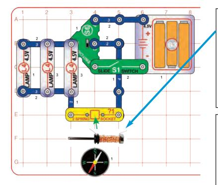
The wire magnet in the preceding circuit is not very powerful because it only has a few loops of wire, but you can make a better one. Assemble the build-your-own electromagnet (the thin wire wrapped around an iron core rod, with the ends connected to the 2-spring socket (?1)) using the instructions on page 5.
