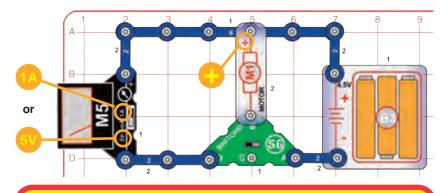
This circuit uses the batteries (B3) to get the motor spinning, then disconnects the batteries and uses the motor as a generator. A **generator** uses mechanical motion (here the spinning motor shaft) to create electricity (a current in a coil in the motor). The meter shows how much current and voltage are produced by the spinning shaft, with and without the fan.
