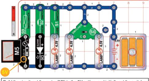
Build the circuit, set the meter (M5) to the 5V setting, and initially set the switcher (S6) to the middle position. Turn on each of the switches:
