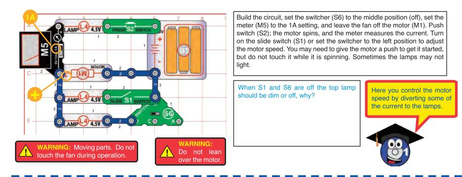
Now place the fan on the motor. Turn on the slide switch and set the switcher to the left (so both switches are on), and push the press switch. The motor will not spin.
