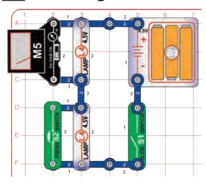
Build the circuit, and set the meter (M5) to the 5V setting. Turn on the slide switch (S1); the lamps (L4) are on and the meter measures the voltage across the top lamp. Push the press switch (S2) to turn off the bottom lamp.
