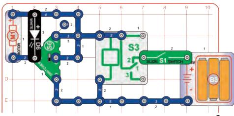
In project 85 and others the LED only works in one of the switcher (S6) settings, but in this circuit it works in either the top or bottom S6 setting. Why?
