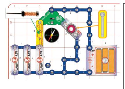
Assemble the build-your-own electromagnet (the thin wire wrapped around an iron core rod, with the ends connected to the 2-spring socket (?1)) using the instructions on page 5. Build the circuit, place the iron core rod in the electromagnet (M3).
