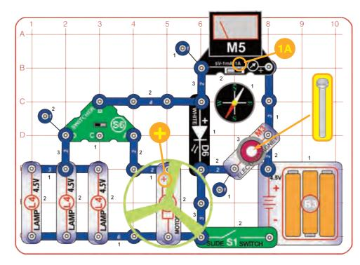
Build the circuit, set the meter (M5) to the 1A setting, place the iron core rod in the electromagnet (M3), and place the fan on the motor (M1). Turn on the slide switch (S1); the white LED (D6) lights, the meter measures the current, and the electromagnet attracts the compass needle. Set the switcher (S6) to the left to the left to light the lamps, to the right to spin the motor & fan, or the middle to do neither.
