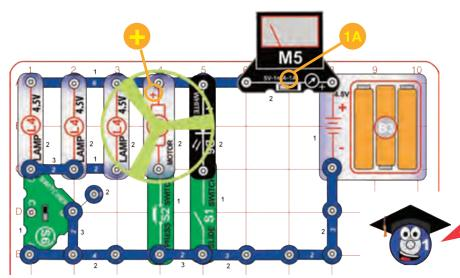
Build the circuit, set the switcher (S6) to the middle or lower position (off), set the meter (M5) to the 1A setting, and place the fan on the motor (M1). Set the switcher to the top position to light the lamps (L4), push the press switch (S2) to spin the motor, and turn on the slide switch (S1) to light the white LED (D6). Try each switch separately and in different combinations, and compare the current measured on the meter.
