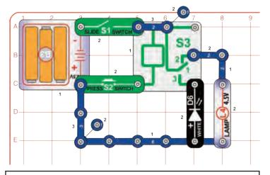
Build the circuit and turn on the slide switch (S1); the lamp (L4) is on. Now push the press switch (S2) to activate the relay (S3); you hear a click as the relay switches power from the lamp to the white LED (D6).
