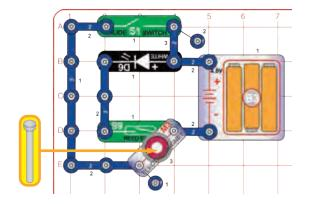
Build the circuit as shown, and turn on the slide switch (S1). The electromagnet (M3) should be activating the reed switch (S9), which turns on the white LED (D6). Raise the iron core rod in the electromagnet (or remove the rod) to turn off the LED.
