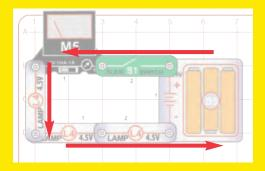
Connecting parts in series is one way of arranging them in a circuit. The advantage of it is that wiring them together is simple. The disadvantage is that if one lamp breaks, all three will be off.
