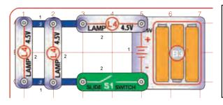
Build the circuit. Turn on the slide switch (S1) on and off several times, watching the brightness of each lamp (L4). Compare the brightness of each lamp, and how quickly each turns on.
