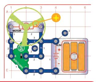
How does electricity turn the shaft in the motor? The answer is magnetism. The motor is the opposite of an electromagnet. Moving a magnet near a coil of wire can make a current flow in it (like the electromagnet), but a current flowing can move a magnet.
