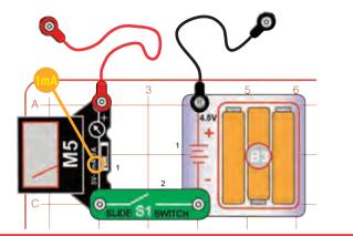
You can use Ohm's Law to measure the resistance of your puddles and drawings. The voltage is about 4.5V. and use the current measured on the meter.
