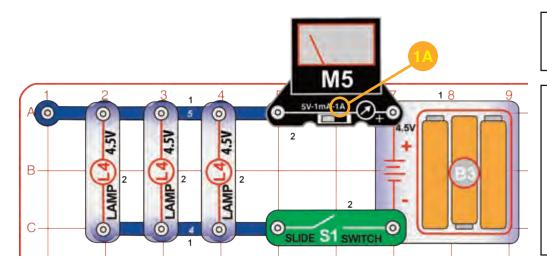
Build the circuit, set the meter (M5) to the 1A setting, and turn on the slide switch (S1). The lamps (L4) are bright and the meter measures the current.
