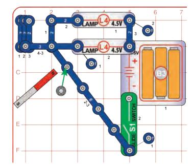
Build the circuit as shown. There are three 2-snap wires at base grid locations A1-B1. Snap the 6-snap wire at base grid location F5, then place it so it lays on the snap at grid location B2 (DO NOT SNAP IT ON). A 3-snap wire is placed across grid locations B1-B3, with the left side on lever 4 and the right side on level 3; sure it is securely snapped. Place the nut snap on the 6-snap wire.
