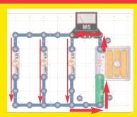
The current from the batteries splits up between the three lamps, because they are connected in parallel. Connecting parts in parallel allows more current to flow, so it decreases the overall circuit resistance.
