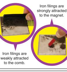
Running the comb through your hair builds up an electric charge in it, which is different from the magnetic charge in the magnet. The paper pieces are attracted to an electric charge, while the iron filings are attracted to a magnetic charge.
