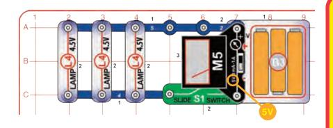
Build the circuit, set the meter (M5) to the 5V setting, but leave the slide switch (S1) off. The meter measures the voltage on the batteries. The lamps (L4) will be off, because the switch is off.
