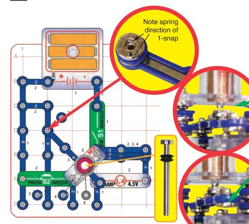
The current through the electromagnet makes a magnetic field that attracts the nut-snap, which breaks the circuit to the lamp.
