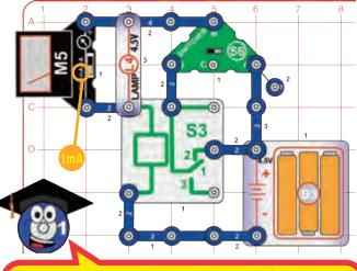
The current is actually more than 1mA (about 50mA when the relay is on continuously), but the lamp is used here to adjust the current to be within the 1mA range on the meter. To see the actual current, remove the lamp and set the meter to the 1A setting; it should be slightly above 0.
