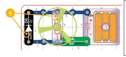
Build the circuit shown and watch the white LED (D6) as you push and release the press switch (S2). Notice that even though the LED is connected backwards, it is flashing dimly while the fan is spinning, and then flashes brightly when you release the press switch.
