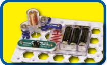
Build the circuit as shown and drop the thin rod into the electromagnet (M3). Push the press switch (S2) several times. The thin rod gets sucked into the electromagnet and can be suspended there, or you can bounce it up and down.
