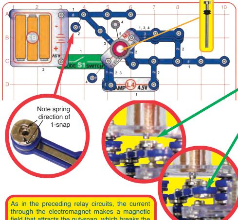
through the electromagnet makes a magnetic field that attracts the nut-snap, which breaks the circuit to the lamp. However in this circuit attracting the nut-snap also breaks the circuit to the electromagnet, which then releases the nut-snap. This creates a feedback loop which raises and releases the nut-snap in a repeating cycle. The buzzing sound you hear is from raising and releasing the nut-snap many times a second.
