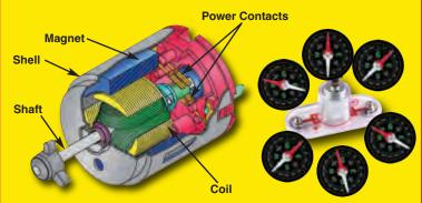
To prove the motor has a magnet inside, move your compass around it. The red needle will be attracted to one side but repelled from the other.
