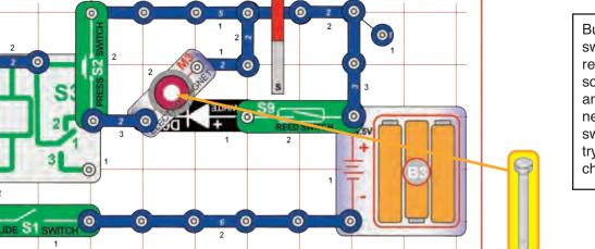
Build the circuit as shown, and turn on the slide switch (S1); you may hear a buzzing sound as the relay (S3) turns on and off rapidly. Adjust the sound by pushing the press switch (S3), raising and lowering the iron core rod in the electromagnet (M3), or by placing the magnet near the reed switch (S9) to activate it and the white LED (D6); try combinations of these and see how the sound changes.
