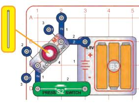
**Note:** the magnet poles may be opposite of how it's shown here, depending on how you connected the *electromagnet* (M3).
