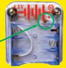
Fuses are designed to shut down a circuit when the current is abnormally high (indicating something is wrong, such as a component failure, bad design, or a person using it improperly). This shutdown prevents further damage to the circuit, and can prevent explosions or fires. Fuses are important for safety and most electrical products have one, especially if they use electricity supplied by your local electric company.
