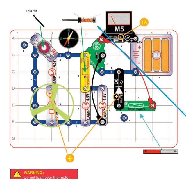
Electronics is the science of working with and controlling electricity. This circuit is shown on the front of the Snap Circuits<sup>®</sup> STEM box, use that picture to help in building it.
