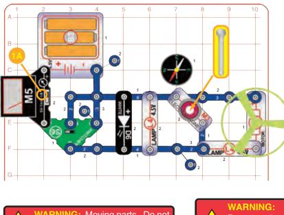
Build the circuit, set the meter (M5) to the 1A setting, place the iron core rod in the electromagnet (M3), and place the fan on the motor (M1). Set the switcher (S6) to the left or right to make electricity flow through the lights, motor, and electromagnet in opposite directions. The compass measures the magnetic field from the electromagnet and the meter measures the current from the batteries. Set the switcher to the middle position to shut off the circuit.
