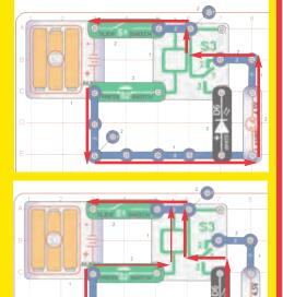
The current through the press switch activates the coil in the relay, which changes the relay connection from contacts 1-2 to contacts 1-3. There is no electrical connection between the relay's coil and 1-2-3 contacts, so those circuits do not affect each other, and can operate at different voltages. In this way a low-voltage circuit can control a high-voltage or high-current circuit.
