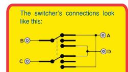
The switcher is used to reverse the battery connections (from snap A & D) to snaps B & C, which reverses the voltage across the motor and lamp. In the top position, battery "+" is connected to snap B, and in the bottom position battery "+" is connected to snap C.
