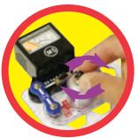
Build the circuit and set the meter (M5) to the 1mA scale. Spin the motor (M1) top clockwise with your fingers and watch how much current is produced. (Clockwise means in the direction in which the hands of a clock rotate.)
