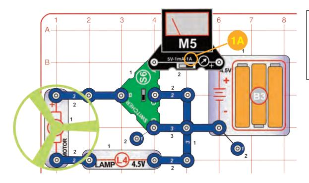
Study the circuit. What will happen to the motor, lamp, and meter if you change the switcher to the bottom position? (Try it.)
