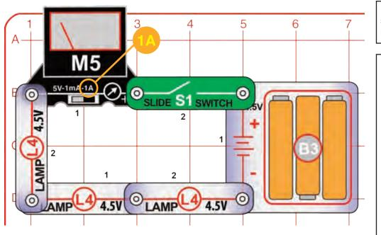
The three lamps are connected in a series, and all the electric current from the batteries flows through each component in the circuit. The lamps are dim because the voltage from the batteries (B3) is divided between them.
