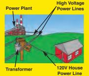
A transformer is a magnetic bridge, since we use magnetism to cross an air gap that electricity cannot cross by itself.
