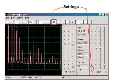
The spectrum at left is for just after pressing the press switch. The spectrum below uses the same settings and shows the spectrum just before the sound stops. The frequencies and amplitude slowly get lower as the sound fades away.
