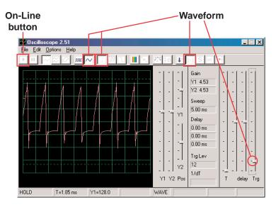
Winscope has a mode that can display multiple scans at the same time, called **Storage mode**. Set the adjustable resistor lever to a low-middle position, place Winscope in this mode, and watch the results.
