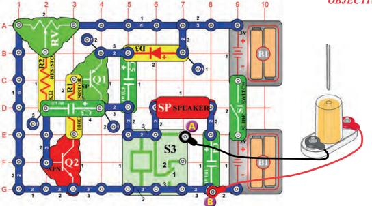
into the electromagnet (M3) center. Connect the electromagnet to points A & B with the jumper wires and hold it about 1 inch above the table. Slide the adjustable resistor (RV) control lever around slowly, you will hear a clicking sound from the relay (S3) and speaker (SP).
