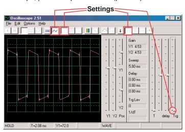
Click on the **5ms/div time scale button** and on the **FFT button** to look at the frequency spectrum for the signal. The Y1 gain control is set for high gain now, so the higher peaks are off the screen but lots of the lower peaks are visible.
