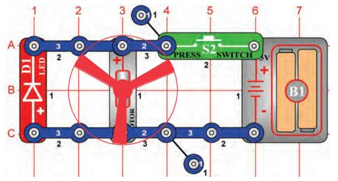
**WARNING:** Moving parts. Do not touch the fan or motor during operation. Do not lean over the motor.
