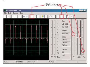
The waveform at left shows the signal just after pressing the press switch, the waveform below uses the same settings and shows the waveform just before the sound stops. You see the pulses slowly spread out as the tone of the sound changes.
