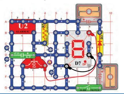
The circuit switches between numbers "3" & "6" on the display. Place a jumper from segment C to segment D and segment B to point A.
