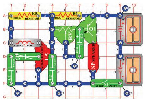
Turn on the slide switch (S1) and adjust the variable capacitor (CV) for a radio station. Make sure you set the variable resistor (RV) control to the left for louder sound.
