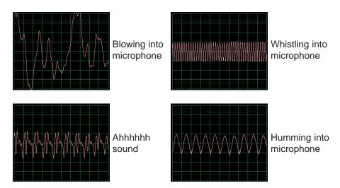
Click on the **FFT button** to look at the frequency spectrum for these signals. Try the **amplitude** and **time scales** shown here to start, but your best settings will depend on what sounds you make, how loud you speak, and how close you are to the microphone.
