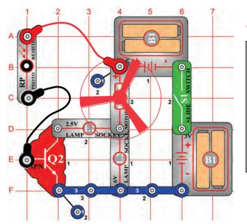
OBJECTIVE: To demonstrate how the motor draws more current to exert greater force when spinning slowly.
