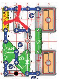
OBJECTIVE: To build a sound activated fan.
