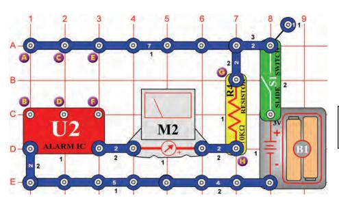
OBJECTIVE: Use the meter with the alarm IC.
