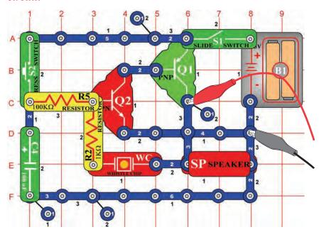
Build the circuit shown. If continuing from the previous experiment then close the Winscope program and run it again, to reset the settings. Click on the On-Line button to activate, turn on the switch (snap part S1), and press the press switch (part S2). Try the **settings** shown here.
