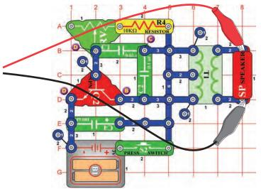
Build the circuit and try the **settings** shown. Start with the adjustable resistor set to the left but then adjust to change the tone. The signal dies out after you release the switch.
