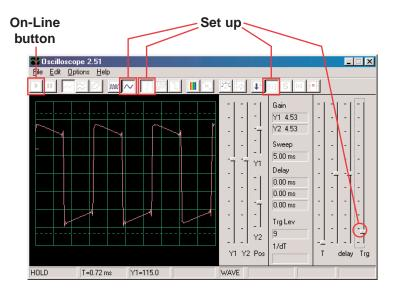
You should see a waveform similar to that shown here, but it will be constantly changing. This is because the siren sound you hear is not a continuous tone but instead is constantly changing. Note the differences in the waveshape for this circuit compared to the circuit in Project PC1.
