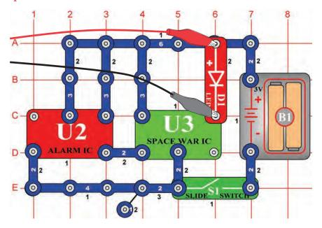
Build the circuit shown. If continuing from the previous experiment then close the Winscope program and run it again, to reset the settings. Click on the **On-Line button** to activate, and turn on the switch (snap part S1). Set Winscope to the **settings** shown below. The signal from the alarm IC (snap part U2) causes the space war IC (part U3) to step through the 8 different patterns it can create. A sample waveform is shown here.
