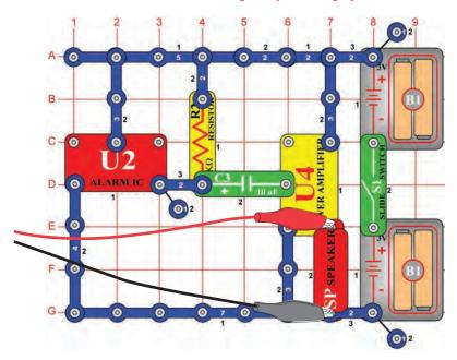
Build the circuit shown and set Winscope to the **settings** shown below. The siren sound is very loud. In most cases the waveform will have **flat edges** on the top and bottom, indicating the voltage is too high for the microphone input stage on your computer and is being distorted. You may sometimes correct for this if you like by reducing the volume control of your microphone input (see p. 3), but it is recommended that you return the volume to the normal level before doing other projects.
