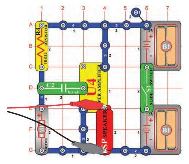
Build the circuit shown. If continuing from the previous experiment then close the Winscope program and run it again, to reset the settings. Click on the On-Line button to activate, and turn on the switch. Set Winscope to the **settings** shown on the upper right. Turn the motor (snap part M1) slowly with your fingers and watch the waveforms generated. They are very erratic and unpredictable. A sample is shown on the upper right.
