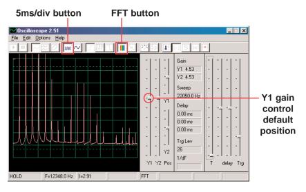
You are seeing the frequency spectrum of your signal, up to 22kHz. Notice that most of the energy is at the low frequencies (below 7kHz), and there is very little as you go higher.
