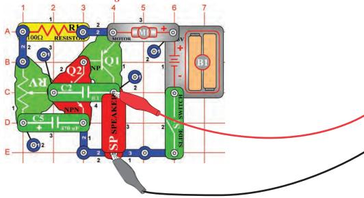
Build the circuit shown. If continuing from the previous experiment then close the Winscope program and run it again, to reset the settings. Click on the **On-Line button** to activate, and turn on the switch (snap part S1). Set Winscope to the settings shown below, and move the lever on the adjustable resistor (snap part RV) around to change **the waveform** and the sound. A sample waveform is shown here, but the pattern and shape of the pulses depends on the adjustable resistor setting.
