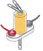
Snap two 2-snaps around a paperclip and lift them with the electromagnet, as shown here on the left.
