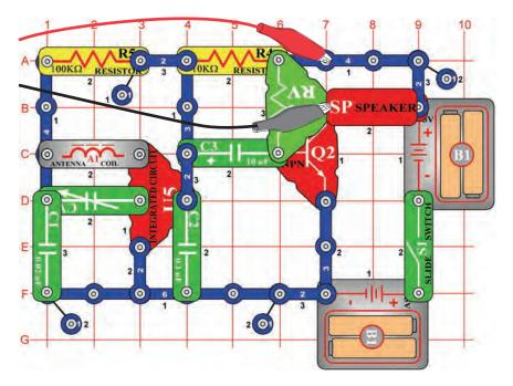
Turn on the switch and adjust the variable capacitor (CV) for a radio station, then adjust the loudness using the adjustable resistor (RV). Use the same Winscope settings as for project PC12 (AM radio) to view the waveform and frequency spectrum. The waveform will be different from that in projects PC12 and PC38, because those circuits use the power amplifier IC (U4) instead of the NPN transistor for amplification.
