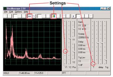
This is the spectrum for the oscilloscope waveform shown on the preceding page, which alternates between pulses and flat. Because of the transition between pulses and flat, the spectrum is the irregular shape shown here.
