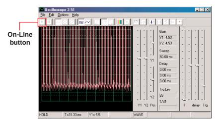
The waveform peak is off the top of the screen because the scope gain (amplification) is set too high. You may adjust this gain by moving the **Y1 gain control** around (try it).
