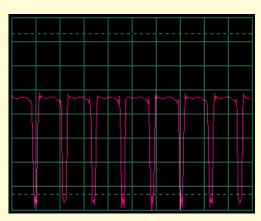
If this is the case then swap the connections of the red and black clips of the Winscope probe in all circuits. C. The shape of waveforms may appear distorted for some circuits, due to protection circuitry that acts as a filter. For example:
