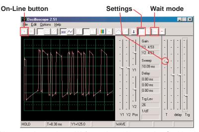
You can also activate **Wait mode** and press the On-Line button several times to view one scan of the signal at a time, instead of seeing continuous scans.
