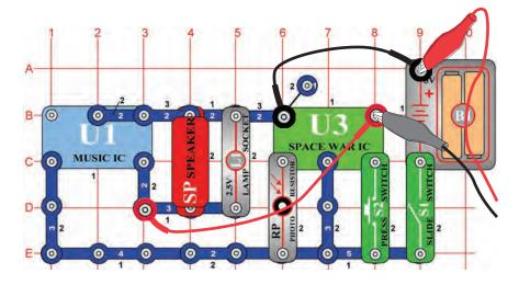
Build the circuit and try the **settings** shown. Turn it on, press the press switch (S2) several times, and wave your hand over the photoresistor (RP) to view all the sound combinations. Compare the waveform and spectrum to the alarm IC combo circuit.
