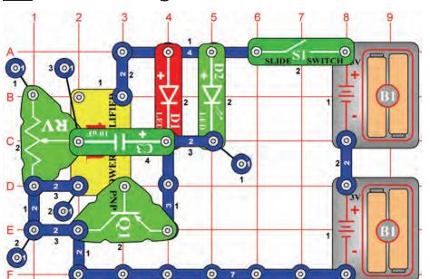
OBJECTIVE: To construct an LED flasher.
