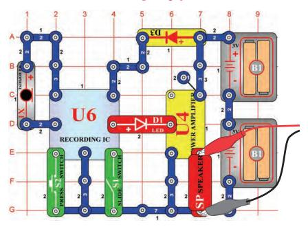
Build the circuit shown. Turn on the slide switch (S1), you hear a beep signaling that you may begin recording. Talk into the microphone (X1) up to 8 seconds, and then turn off the slide switch (it also beeps after the 8 seconds expires).
