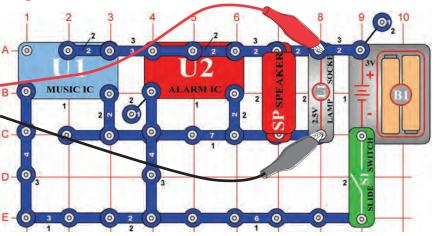
Build the circuit and try the **settings** shown. Turn it on and view the waveforms.
