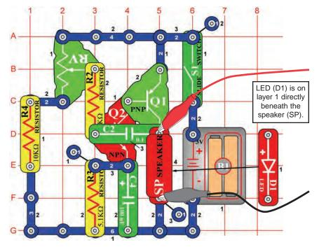
Build the circuit shown. If continuing from the previous experiment then close the Winscope program and run it again, to reset the settings. Click on the On-Line button to activate, and turn on the slide switch (snap part S1). Set Winscope to the **settings** shown on the upper right, and move the lever on the adjustable resistor (snap part RV) around to change the waveform and the sound. At some positions there may be no sound. A sample waveform is shown on the upper right.
