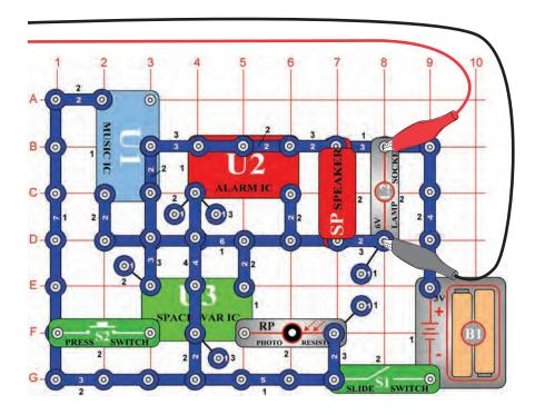
The Symphony of Sounds project combines waveforms from the Music, Alarm, and Space War integrated circuits. Build the circuit shown. If continuing from the previous experiment then close the Winscope program and run it again, to reset the settings. Click on the On-Line button to activate, and turn on the switch (snap part S1). Press the press switch (S2) and wave your hand over the photosensitive resistor (RP).
