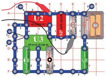
Build the circuit and try the settings shown. Turn it on, press the press switch (S2) several times, and wave your hand over the photoresistor (RP) to view all the sound combinations. You may also use FFT mode to view the frequency spectrum.
