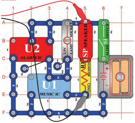
Build the circuit shown. If continuing from the previous experiment then close the Winscope program and run it again, to reset the settings. Click on the On-Line button to activate, and turn on the slide switch (snap part S1). Try the **settings** shown here.
