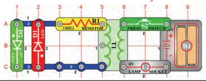
Watch the LED's (D1 & D2) as you press or release the press switch (S2). The red LED (D1) lights briefly just as you press the press switch and the green LED (D2) lights briefly just after you release it, but neither lights while you hold the press switch down. Why?
