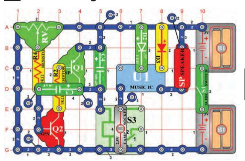
Set the adjustable resistor (RV) to the far left position and turn the slide switch (S1) on. The relay's (S3) contacts open and close shorting U1 to ground, causing the sound level to change.
