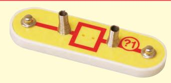
The two-spring socket (?1) just has two springs, and won't do anything by itself. It is not used in any of the experiments. It was included to make it easy to connect other electronic components to your Snap Circuits®. It should only be used by advanced users who are creating their own circuits.
