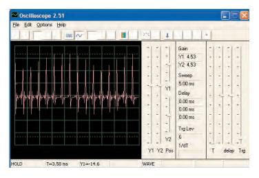
Winscope makes measurements using a 44kHz sampling rate, which is fast enough to measure the frequency of this signal (varying from 1-5kHz). However these pulses have much of their energy spread among higher frequencies that approach the sampling rate (see the sample spectrum plots at right), where the amplitude measurement becomes increasingly inaccurate.
