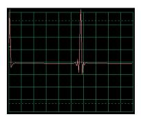
The waveform above is weak and erratic, so replace the  $0.02\mu F$  capacitor (snap part C1) with the  $0.1\mu F$  capacitor. A sample of the new waveform is at left, with the same settings. It is lower in frequency but higher in amplitude.
