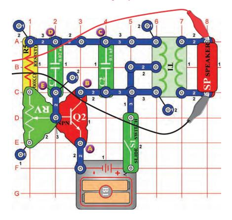
Build the circuit and try the **settings** shown. Move the adjustable resistor lever to change the pitch of the sound and pulse separation in the waveform.
