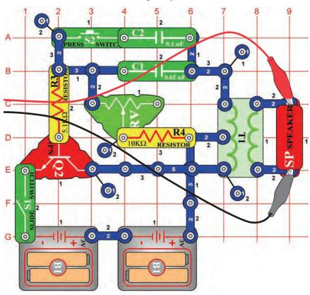
Build the circuit and try the settings shown. Flip on the slide switch and press the press switch a few times while moving the adjustable resistor control around. View the waveform and frequency spectrum.
