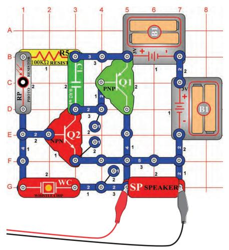
Build the circuit shown. If continuing from the previous experiment then close the Winscope program and run it again, to reset the settings. Set Winscope to the **settings** shown below and click on the On-Line button to activate. A sample waveform is shown here.
