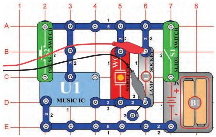
Build the circuit shown. If continuing from the previous experiment then close the Winscope program and run it again, to reset the settings. Click on the On-Line button to activate, and turn on the slide switch (snap part S1). Try the **settings** shown here. When the music stops, press the press switch (part S2) and it will resume.
