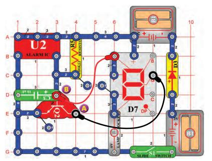
The circuit switches between letters "c" & "C" on the display. Place a jumper from point A to segment G and point B to segment A.
