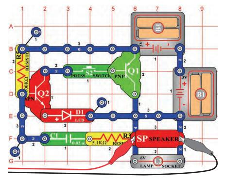
Build the circuit shown. If continuing from the previous experiment then close the Winscope program and run it again, to reset the settings. Click on the On-Line button to activate, and hold down the press switch (snap part S2). Set Winscope to the **settings** shown on the upper right. A sample waveform is shown on the upper right.
