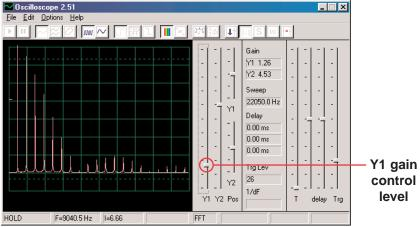
Move the adjustable resistor control (snap part RV) and watch how it changes the frequencies on the display.
