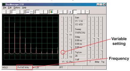
As you can see, all the peaks are equally spaced in frequency. Move your computer mouse directly over the first peak, the software displays the **frequency** you are pointing at. Move the mouse to the other peaks and you see they are multiples of the first frequency.
