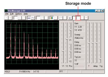
In this way you can show the peak energy achieved at each frequency. But this is only useful on a stable waveform, so if you move the adjustable resistor lever now the signal will fill the screen as the peaks move across the display.
