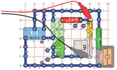
Use the LOW (or 10mA) setting on the meter (M2). Set the adjustable resistor (RV) to the bottom position and turn on the slide switch (S1), you will see a waveform like that shown below. Set the adjustable resistor to the top, and the waveform looks like that shown on the bottom left, due to lower resistance in the circuit. A sample frequency spectrum is also shown on the bottom right.
