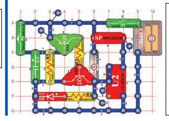
Replace the 1-snap wire from the middle snap on U2 with a 2-snap and connect it to grid location D7 & E7. The circuit now produces a different sound. Change R5 and C5 with the following combinations for R5 and C5:
