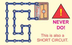
When the slide switch (S1) is turned on, this large circuit has a SHORT CIRCUIT path (as shown by the arrows). The short circuit prevents any other portions of the circuit from ever working.
