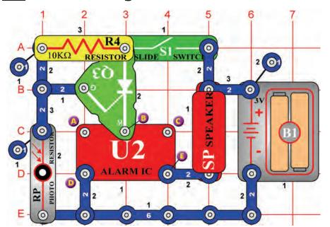
As the photoresistor (RP) is exposed to light, its resistance is very low, thereby connecting the gate of the SCR (Q3) to ground. This prevents the SCR from conducting, connecting the alarm IC (U2) to the batteries. The alarm IC remains off until the light is blocked, triggering the SCR. If the light in the room is not bright, the IC may turn on.
