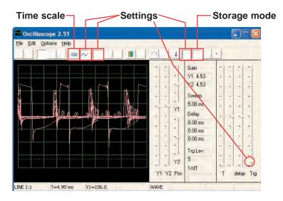
You may replace the  $0.02\mu F$  capacitor C1 with  $0.1\mu F$  capacitor C2 or  $10\mu F$  capacitor C3 ("+" on the right) to change the sound, but you may want to change the **time scale**.
