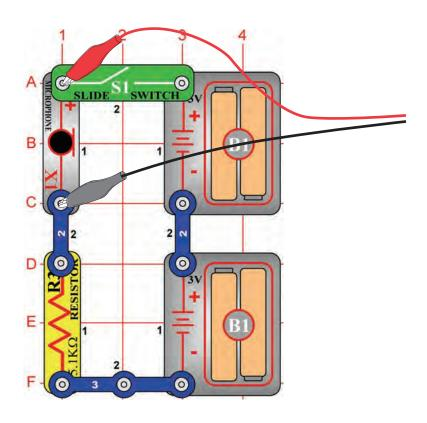
If continuing from the previous experiment then close the Winscope program and run it again, to reset the settings. Click on the **On-Line button** to activate Winscope, and turn on the switch (snap part S1).
