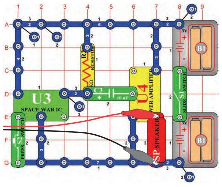
Build the circuit shown and use the same settings as in PC31 to view the waveform. Press the switch (S2) to change the sounds and waveform.
