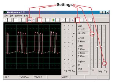
The oscilloscope display alternates between 2 waveforms, the one shown here and the one on the next page. This one shows some pulses followed by a flat signal, then more pulses, then flat, then pulses, then flat . . .
