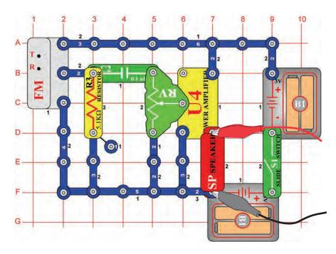
Turn on the slide switch (S1) and press the R button. Now press the T button and the FM module scans for a radio station. When a station is found, it locks on to it and you hear it on the speaker. Press the T button again for the next radio station.
