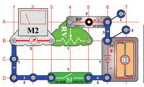
Set the meter (M2) to the LOW (or 10mA) setting. Using only a few parts, you can make a simple light meter. The amount of light changes the resistance of the photoresistor (RP), which affects the current though the meter. As light increases, the resistance drops and the meter deflects to the right. Decreasing the light, the meter deflects to the left, indicating less current.
