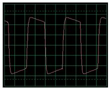
Typical waveform using 0.02µF capacitor
