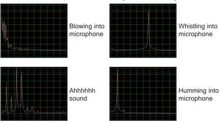
The above frequency spectrum pictures correspond directly to the waveform pictures on the preceding page. Notice that the spectrums for the hum and whistle have only a single big peak. Smooth, well-rounded, and repetitive waveforms (in oscilloscope
