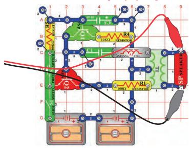
Build the circuit and try the **settings** shown. Flip on the slide switch and press the press switch for a few seconds and release. View the waveform as a siren starts up and then slowly fades away.
