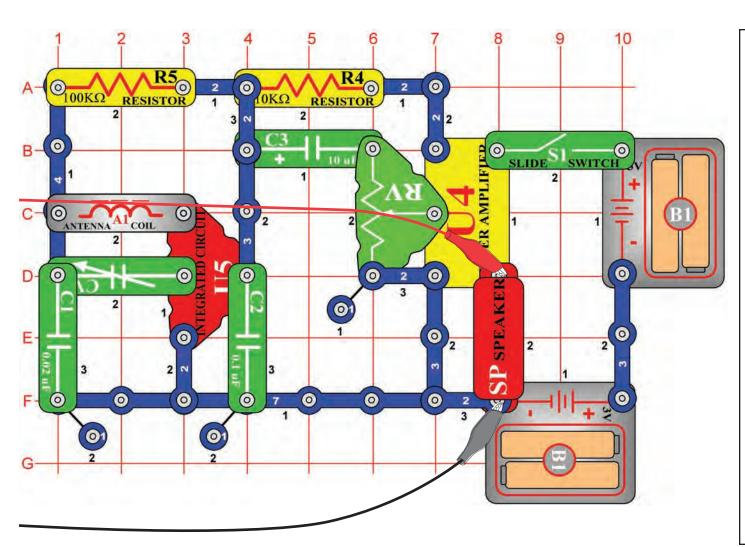
Build the circuit shown and connect the PC-interface cable to the microphone input on your computer. Turn on the slide switch (snap part S1), tune the variable capacitor (snap part CV) to a local radio station that gives good reception, and set the adjustable resistor (snap part RV) to a comfortable volume. The integrated circuit (snap part U5) detects and amplifies the AM radio waves all around you. The power amplifier IC (snap part U4) drives the speaker (snap part SP) to complete the circuit.
