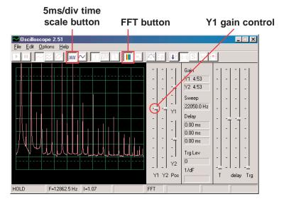
Note that the sound is music and the oscilloscope waveform has a "square" shape, as a result the frequency spectrum has a lot of peaks with equal spacing.
