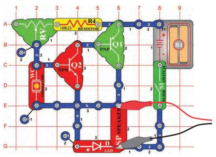
Build the circuit shown, and try the **settings** below. Move the adjustable resistor lever to change the frequency. A sample waveform is shown here.
