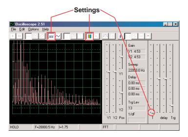
Note that in the above display the Y1 Gain is set high to show the low energy levels of the higher frequency components of the signal, even though the stronger peaks of the lower frequency components are off the top of the display. This can be deceiving. Now change the Y1 Gain so that the highest peak can be seen, this is shown on the right. Now you see how the main signal frequency dominates the others.
