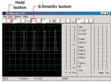
With the time scale at 0.5ms/div and the adjustable resistor set for middle position, you should now have a picture similar to this one.
