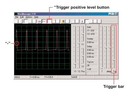
The small slash "-" represents the trigger voltage, when the signal reaches this voltage level it activates the display. This makes it easy to observe a stream of pulses like you have now, and also to record a single (non-repeating) pulse.
