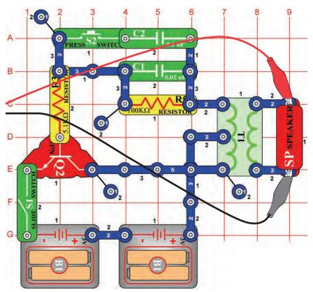
Build the circuit and try the **settings** shown. Press the press switch to lower the frequency of the signal by increasing the capacitance in the oscillator. You can replace the  $0.1\mu F$  capacitor C2 with the  $10\mu F$  capacitor C3 ("+" on the right) to further lower the frequency of the tone. You may try other settings to zoom in or look at the frequency spectrum.
