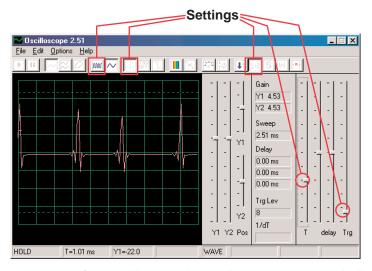
The actual waveform will vary depending on how much light is shining on the photoresistor (snap part RP). If you cover the photoresistor then the circuit shuts off.
