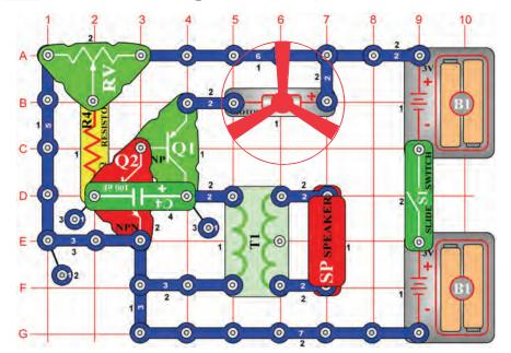
Adjust the adjustable resistor (RV) to the middle position and turn on the slide switch (S1). As the circuit oscillates, the motor (M1) moves a short distance as the speaker (SP) sounds. Adjust the adjustable resistor to different positions seeing how it affects the motor and speaker.
