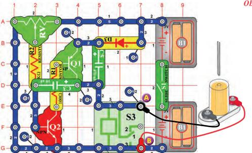
Take a paperclip and straighten it out, bend it in half, and place it into the electromagnet (M3) center. Connect the electromagnet to points A & B with the jumper wires and hold it about 1 inch above the table. Slide the adjustable resistor (RV) control lever around slowly, you will hear a clicking sound from the relay (S3).
