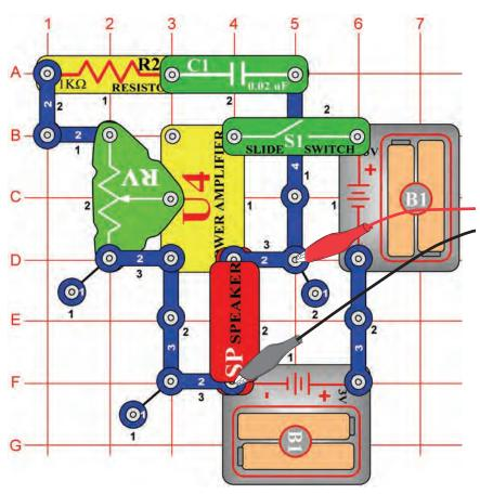
Build the circuit shown. If continuing from the previous experiment then close the Winscope program and run it again, to reset the settings. Click on the On-Line button to activate, and turn on the switch (snap part S1). Set Winscope to the **settings** shown below, and move the lever on the adjustable resistor (snap part RV) around to change the waveform and the sound. At some positions there may be no sound. A sample waveform is shown here.
