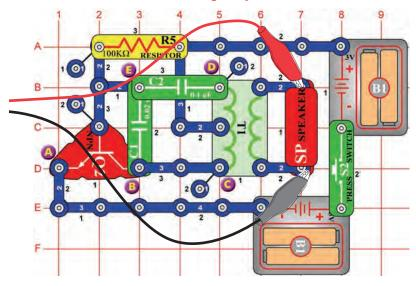
Build the circuit and try the **settings** shown here. This circuit produces a series of pulses (shown below), representing when the transistor is activated.
