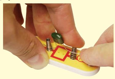
Any component with two wires coming from it (called leads) can be connected with the two-spring socket (?1), assuming the leads are long enough. Usually you will connect different values of resistors or capacitors, but other components like LED's, diodes, or coils/inductors can also be used. You can usually find electronic components at any store specializing in electronics.
