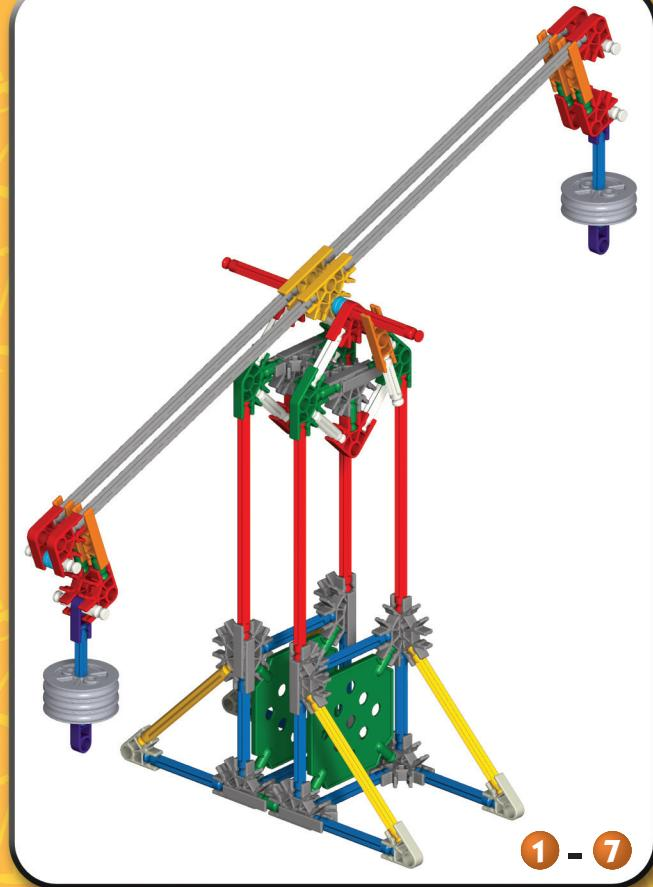
A balance is a 1<sup>st</sup> class lever. It weighs things like letters and apples. To make a balance work, you put the thing to weigh (the resistance) on one side, and weights (the effort) on the other. The fulcrum is in the middle. When the objects equal the same amount, the balance arm will be perfectly straight (level). If you move the resistance close to the fulcrum, you need less effort to balance it.
