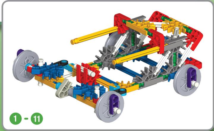
The steering wheel in a car is a wheel and axle. The steering wheel does not actually turn the tires of the car. It turns the steering column (the axle) that works with the machinery inside the car to turn the wheels. It would be very hard to turn the small steering column itself while driving. The steering wheel needs less force to turn it but you have to turn in a bigger circle.
