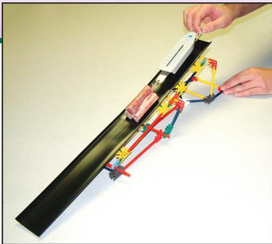
Ramps are inclined planes – sloped, flat surfaces that may or may not be smooth. When you move an object along an inclined plane, you use less force than if you lifted it straight up or put it straight down. However, you have to travel a longer distance to get it to the same place. The longer the ramp, the less force you need to do the job.
