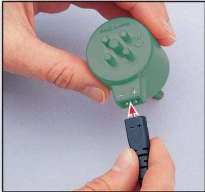
1. Plug the Power Cord fully into the Motor Jack matching the polarity on the Plug and Jacks.
