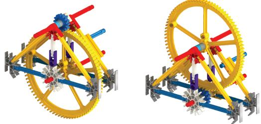
(c) Think of a way to compare the speed that the fan turns, with the speed of the crank when the big gear is attached to the crank and the small gear is attached to the fan blades.
